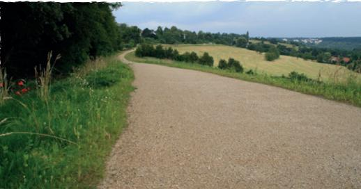
The Stabilizer ECO binder is used to create high-quality and highly functional coverings in the water-bound construction method. These stabilizer surfaces are considered unsealed surfaces and positively support climatic situations in cities and communities. Surfaces containing Stabilizer ECO binders show high strength and long durability while featuring a high water permeability. In addition, the coverings bind dust. Moisture is bound in the coating and metered to the atmosphere.
