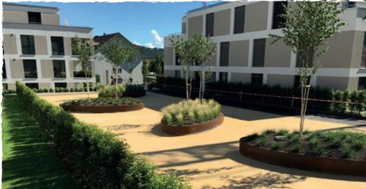
With StaLok you get a hard top layer, which is still permeable to water and air. The mineral mixtures are solidified by a co-polymere. Usage of the the cover layer increases the shear strength and load capacity in wet and dry conditions. Especially during frost and deicing salt periods this binder gives you better surface hardness, allowing a more versatile use of road surfaces.
